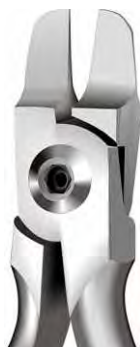
Tweed WI-12-4611 T/C 11.5 cm/ 4½" Rectangular Arch Pliers, Tweed Style Forming plier for square or rectangular wires. The blades are designed to be parallel at .020" ( 0.51 mm) opening. The working edges are carefully diamond-honed to prevent wire scoring.
