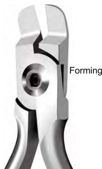
Tweed WI-12-4611 T/C 11.5 cm/ 4½" Rectangular Arch Pliers, Tweed Style Forming plier for square or rectangular wires. The blades are designed to be parallel at .020" ( 0.51 mm) opening. The working edges are carefully diamond-honed to prevent wire scoring.
