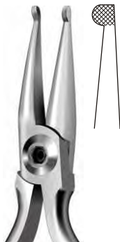
How WI-12-4913 13 cm/ 5¼" Utility Plier , How Long well tapered shape, With 3/32" ( 2.4mm) gripping pads which are serrated and shaped , so that their centre line coincides with the axis of rotation of the plier and holds the wire securely. Beaks are rounded to be completely lip safe.
