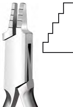
WI-12-6612 Loop Closing Plier, Nance Style Box joint with 4 sectioned tip for forming various size loops in rectangular and round wires. For wires up to .028" ( 0.71 mm).
